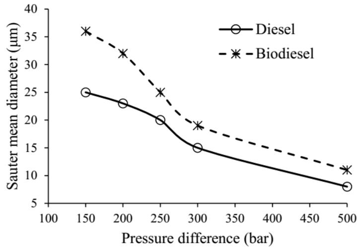
Figure 9. Sauter mean diameters (SMD) in terms of injection pressures
