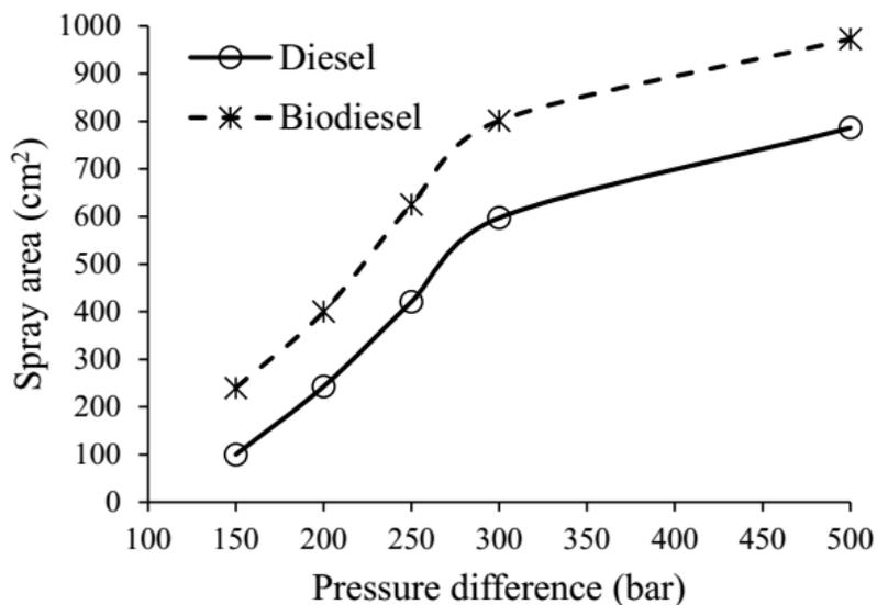
Figure 8. Spray areas in terms of injection pressures
