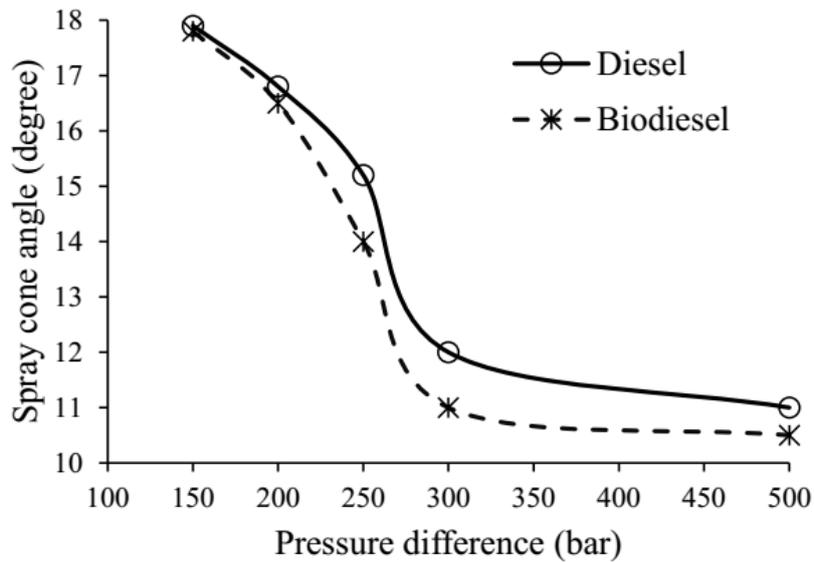
Figure 7. Spray cone angles in terms of injection pressures
