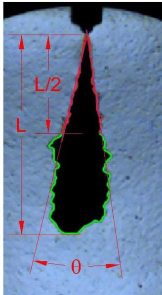
**Figure 4.** Spray tip penetration (L) and spray cone angle ( $\theta$ )
