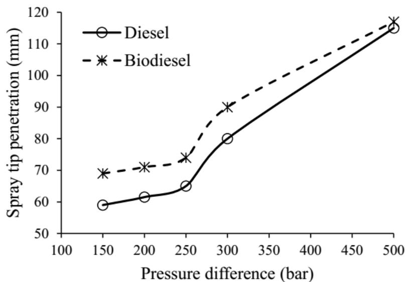
Figure 6. Spray tip penetrations in terms of injection pressures
